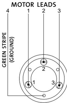
**NOTE:** For Tefzel motor lead, use the following wiring pattern: 1, 2, 3 clock wise from ground terminal (striped green).
