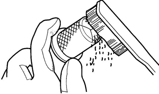
4. Inspect the screen for breaks or tears and replace it if necessary.
