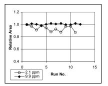
Figure 41 Peak Area Stability for Acrylonitrile
