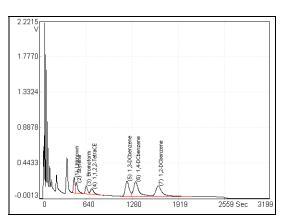
Figure 19 Column A Compounds on the PID
