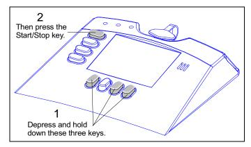
Figure 18 Configuring Voyager to Receive Firmware
