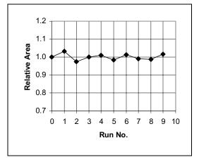
Figure 52 Peak Area Stability for Repetitive Sampling of 11 ppm  $\alpha$ -Pinene
