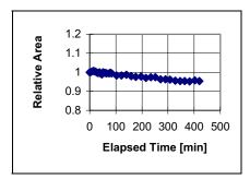
Figure 34 Peak Area Stability for Repetitive Sampling for 100 ppm Isobutylene
