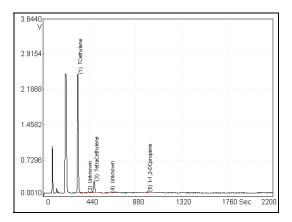
Figure 22 Column B Compounds on the ECD
