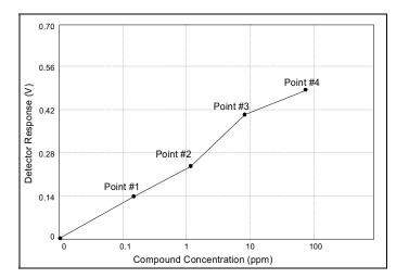
Figure 12 Line Segment Calibration Curve
