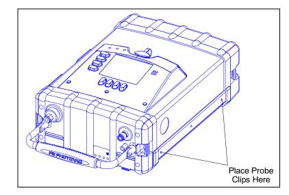
**Figure 4 Placement of Plastic Probe Clips**
