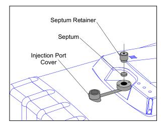
Figure 15 Replacing Septum
