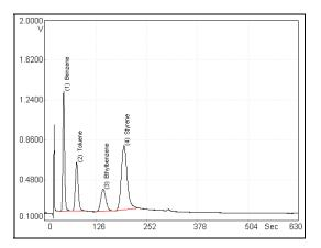
Figure 36 Styrene and Possible Interference Compounds
