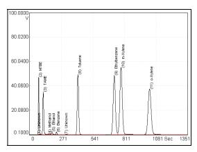
Figure 27 Assay 2 Compounds Run on Column B
