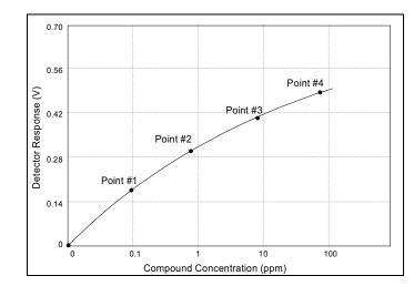
Figure 7 Quadratic Calibration Curve
