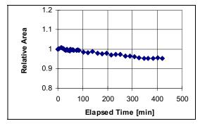
The resulting area drift over a period of 400 minutes is shown in Figure 44. The change in peak area over this time period was 5%.
