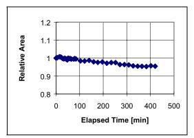
Figure 53 Peak Area Stability for Repetitive Sampling for 100 ppm Isobutylene
