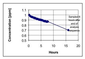
Figure 48 Gas Bag Effect as Measured on a 1 ppm Styrene Sample
