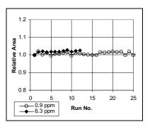
Figure 43 Peak Area Stability for Styrene
