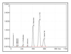
Figure 24 Column C Compounds on the ECD
