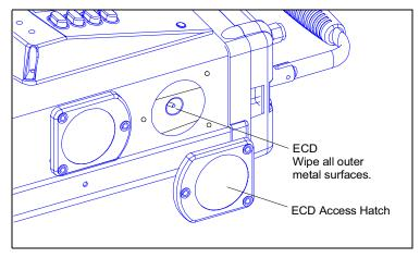
Figure 16 Access to ECD for Wipe Testing
