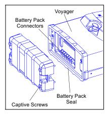
**Figure 2 Removing Battery Pack**
