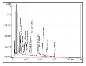
Figure 21 Column B Compounds on the PID
