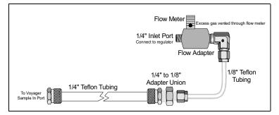
Figure 9 Connecting the Calibration Flow Adapter
