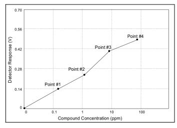
**Figure 6 Linear Calibration Curve**
