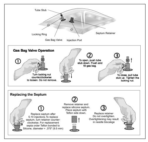
Figure 11 Using the Gas Bag
