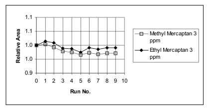
Figure 51 Peak Area Stability for Repetitive Sampling of 3 ppm Methyl Mercaptan and 3 ppm Ethyl Mercaptan
