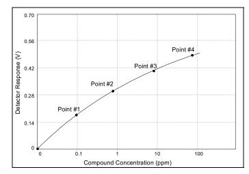
Figure 14 Quadratic Calibration Curve
