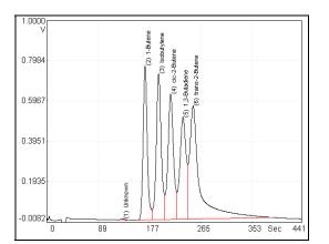
Figure 39 1,3-Butadiene and C4 Interferences
