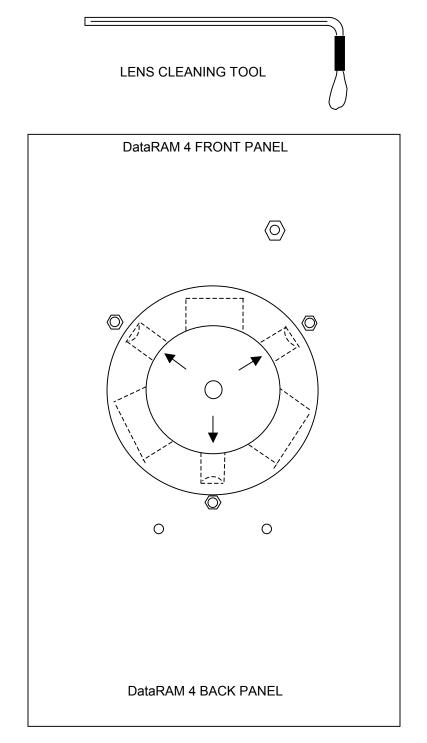
Fig. 5. Lens cleaning tool and bottom view of open filter cavity showing location of sensor chamber lens cavities (arrows).
