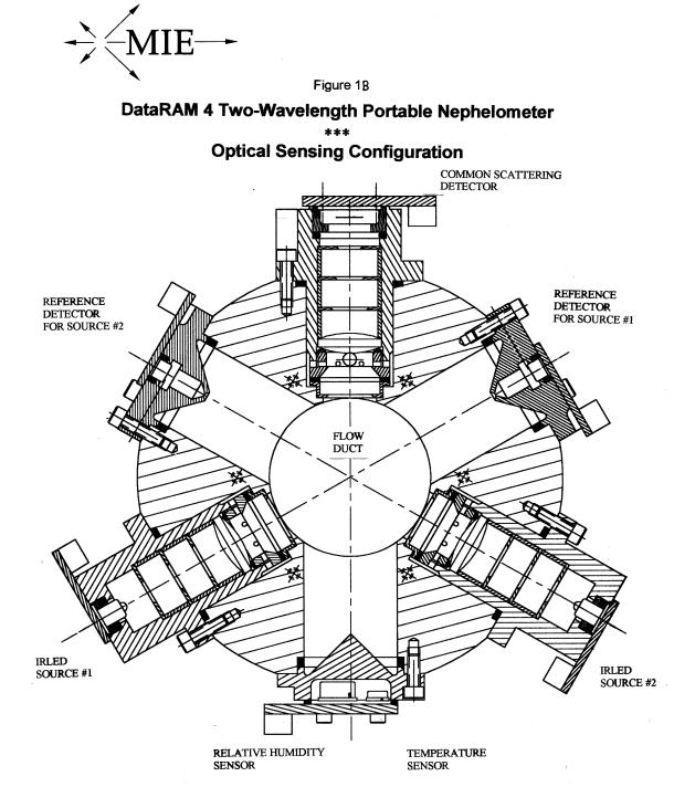
After these two beams traverse the sensing region within the flow duct, they enter their respective light traps at the end of which there are corresponding reference detectors that sense the intensity of each of the illumination beams. Feedback circuits ensure that the light output of both sources remains constant.
