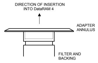
Figure 4. Analytical filter holder with adapter annulus inserted
