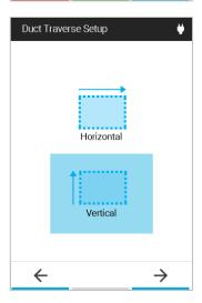
After selecting the traverse orientation (or after selecting a circular duct), the **Insertion Depths** screen will be shown. Note these insertion depths before proceeding.
