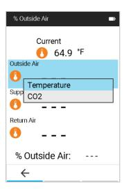
The **Percent Outside Air** feature offers the choice between using Temperature or CO<sub>2</sub> for the Percent Outside Air study if a probe that supports either CO<sub>2</sub> or Temperature is plugged in.
