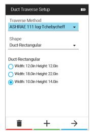
After pressing  $\stackrel{+}{-}$  to add a new duct size, you are brought to the **Flow Setup** page. To change the dimensions, use the arrow keys to navigate between Width and Height then press  $\stackrel{-}{-}$  to begin editing the numbers by using the arrow keys. Press  $\checkmark$  to save the new duct size.
