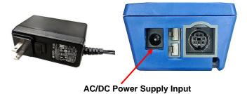
When the AC/DC power supply is connected, the instrument will automatically turn **ON**. To turn the instrument off, disconnect the AC/DC power supply. If batteries are installed, press the power button for 3 seconds.
