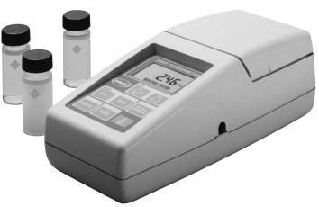
The Hach 2100P and 2100P IS Portable Turbidimeters bring laboratory-level performance on-site, offering fast, accurate results and the ease-of-use analysts demand in the field. With a measurement range of 0 to 1000 NTU and a resolution of 0.01 NTU, the 2100P turbidimeter is ideal for regulatory monitoring, process control or field studies.
