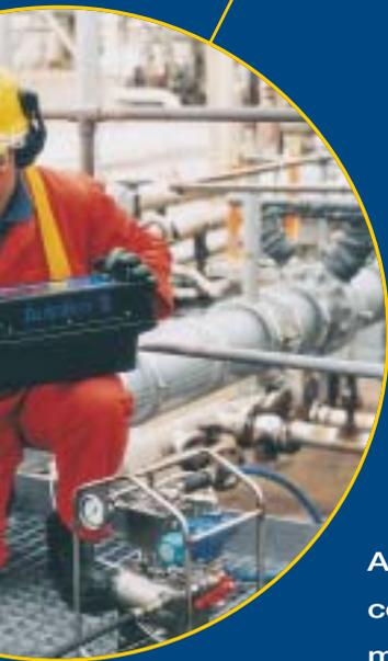
The system can operate for over 40 hours without changing the batteries or cylinder. However, replacement of these in the field is a simple operation for remote or extended use.
