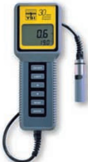
**The YSI 30 instrument** measures salinity, conductivity, and temperature with a super-stable 4-electrode conductivity cell and user-selected scale or autoranging for conductivity. Also available is the YSI 30M with a 50-reading memory with ID. 10-, 25-, and 50-foot cables (3, 7.6, 15.2 m).
