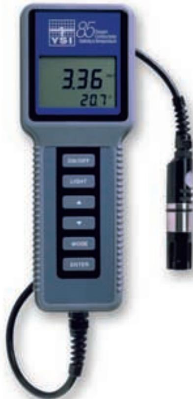
**The YSI 85 multiparameter instrument** offers simultaneous dissolved oxygen, conductivity, salinity, and temperature measurement. For data logging applications, the unit stores up to 50 data sets in non-volatile memory with ID. Features include easy-to-install, screw-on cap membranes, automatic salinity compensation for DO, autoranging for fast, accurate conductivity measurement, and a super-stable 4-electrode conductivity cell. 10-, 25-, 50-, and 100-foot cables (3, 7.6, 15.2, 30.5 m).
