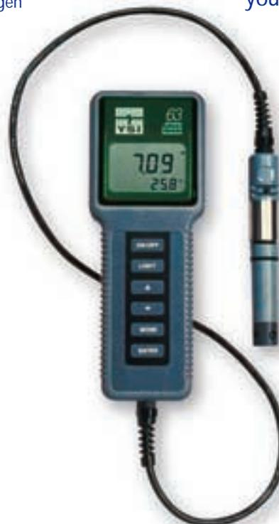
**The YSI 63 instrument** measures temperature, pH, conductivity, and salinity with 50-reading memory with ID, super-stable 4-electrode conductivity cells, field-replaceable pH electrode, a 2-year warranty (pH electrode module, 1-year), user-selected scale or autoranging for conductivity, and up to 100-foot cable due to YSI's Driven-Guard technology. 10-, 25-, 50-, and 100-foot cables (3, 7.6, 15.2, 30.5 m).
