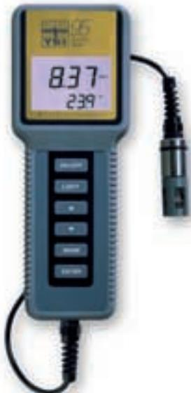
**The YSI 95 instrument** utilizes YSI's patented Microelectrode Array™ (MEA) dissolved oxygen sensor, eliminating the need for stirring during measurement. Features include temperature and salinity compensation, cap membranes for easy replacement in the field, non-volatile memory for storage of 50 data points, and electronic filters to prevent unstable readings. 10-, 25-, 50-, and 100-foot cables (3, 7.6, 15.2, 30.5 m).
