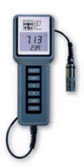
The YSI 60 instrument measures temperature and pH with field-replaceable pH electrode, 50-reading memory, batteries, a 2-year warranty (pH electrode module, 1-year), and up to 100-foot cable due to YSI's Driven-Guard technology. 10-, 25-, 50-, and 100-foot cables (3, 7.6, 15.2, 30.5 m).
