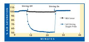
YSI's Microelectrode Array™ (MEA) dissolved oxygen sensor (available on the YSI 95) is an array of very small electrodes, giving it a much smaller surface area than conventional cathodes. Although it maintains the sensitivity of a standard Clark electrode, the MEA sensor is stirring independent and consumes less oxygen
