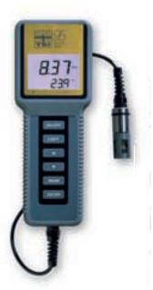
The YSI 95 instrument utilizes YSI's patented Microelectrode Array™ (MEA) dissolved oxygen sensor, eliminating the need for stirring during measurement. Features include temperature and salinity compensation, cap membranes for easy replacement in the field, non-volatile memory for storage of 50 data points, and electronic filters to prevent unstable readings. 10-, 25-, 50-, and 100-foot cables (3, 7.6, 15.2, 30.5 m).
