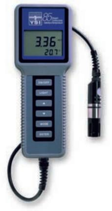
The YSI 85 multiparameter instrument offers simultaneous dissolved oxygen, conductivity, salinity, and temperature measurement. For data logging applications, the unit stores up to 50 data sets in non-volatile memory with ID. Features include easy-to-install, screw-on cap membranes, automatic salinity compensation for DO, autoranging for fast, accurate conductivity measurement, and a superstable 4-electrode conductivity cell. 10-, 25-, 50-, and 100-foot cables (3, 7.6, 15.2, 30.5 m).
