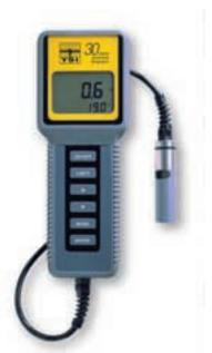
The YSI 30 instrument measures salinity, conductivity, and temperature with a super-stable 4-electrode conductivity cell and user-selected scale or autoranging for conductivity. Also available is the YSI 30M with a 50reading memory with ID. 10-, 25-, and 50-foot cables (3, 7.6, 15.2 m).
