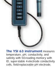
temperature, pH, conductivity, and salinity with 50-reading memory with ID, super-stable 4-electrode conductivity cells, field-replaceable pH electrode, a 2-year warranty (pH electrode module, 1-year), user-selected scale or autoranging for conductivity, and up to 100-foot cable due to YSI's Driven-Guard technology. 10-, 25-, 50-, and 100-foot cables (3, 7.6, 15.2, 30.5 m).
