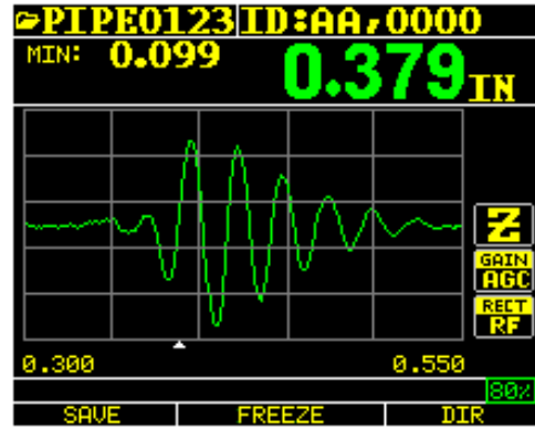
RF signal with cursor upside down "V" indicating where the measurement is being made
