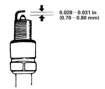
5. Install the spark plug carefully, by hand, to avoid cross-threading.
