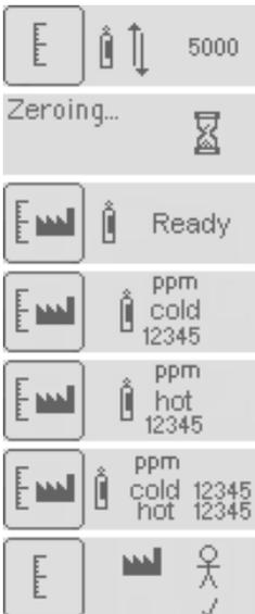
\* Fill an empty (uncontaminated) sample bag with 5000 ppm Helium gas before starting the calibration procedure. Also remove the outer grey probe from the GasCheck Tesla.
