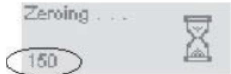
Once the Zero routine is complete the instrument displays it's running screen and is ready for use.
