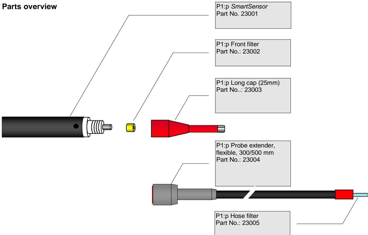
The **ISM** front filter optimises the replacement process for the suction filter as well as the service life of the SmartSensor, which essentially depends on the amount of contamination from the ambient air flowing into the ionisation chamber.
