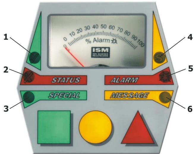
Six LEDs are provided to indicate the different operating modes:
