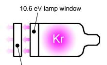
Additional 10.0 eV lamp window mounted in the electrode stack
