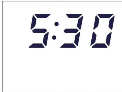
Figure 10: COUNT mode operation showing COUNT Timer of 5 minutes, 30 seconds.
