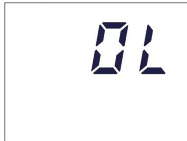
Figure 7: Detector Overload Alarm; will also flash.
