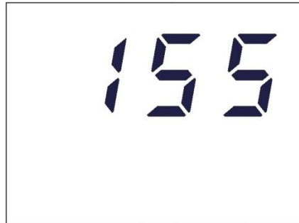
Figure 4: Startup display for Optional Data Logging firmware, showing 155 stored records.
