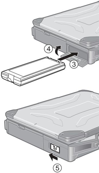
③ Slide the battery pack inward until it is firmly in place.
