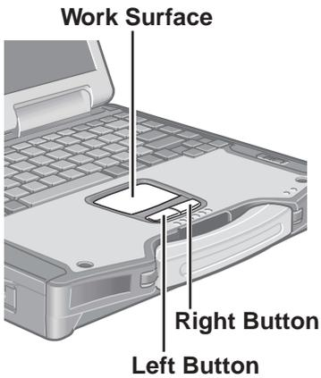
Use the touch pad to move the cursor on the screen and perform computer operations. For instructions on how to operate, refer to <sup>Reference Manual</sup> "Touch Pad".
