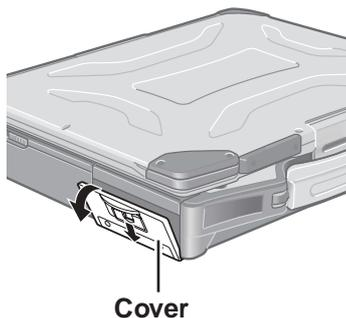
② Slide the latch down, and then without releasing it, open the cover as illustrated.
