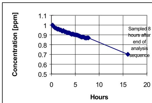
**Figure 48 Gas Bag Effect as Measured on a 1 ppm Styrene Sample**
