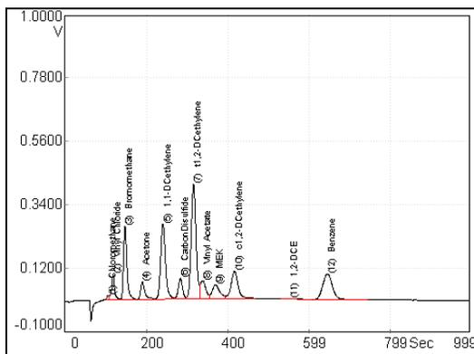
**Figure 23 Column C Compounds on the PID**
