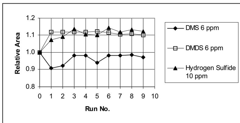
**Figure 49 Peak Area Stability for Repetitive Sampling of 6 ppm DMS, 6 ppm DMDS and 10 ppm Hydrogen Sulfide**
