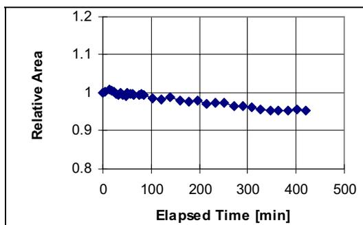
**Figure 44 Peak Area Stability for Repetitive Sampling for 100 ppm Isobutylene**
