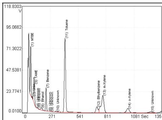
**Figure 28 Gasoline as Run on Column B**
