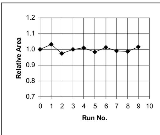
**Figure 52 Peak Area Stability for Repetitive Sampling of 11 ppm  $\alpha$ -Pinene**
