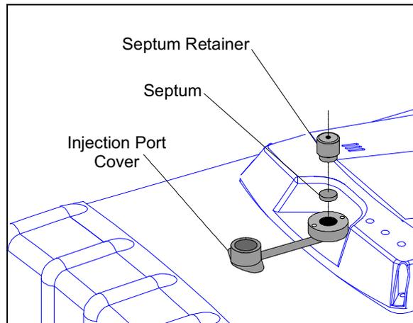
**Figure 15 Replacing Septum**
