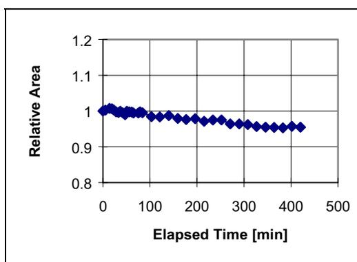
**Figure 53 Peak Area Stability for Repetitive Sampling for 100 ppm Isobutylene**
