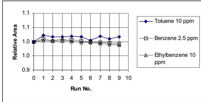
**Figure 32 Peak Area Stability for Repetitive Sampling of 10 ppm Toluene, 2.5 ppm Benzene and 10 ppm Ethylbenzene**
