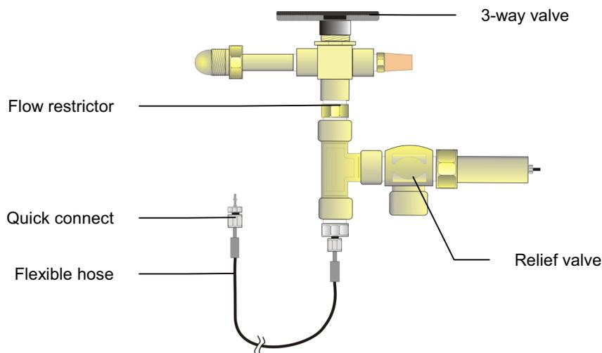
**Figure 3 Carrier Gas Refill Adapters (CGA 590 and CGA 580)**
