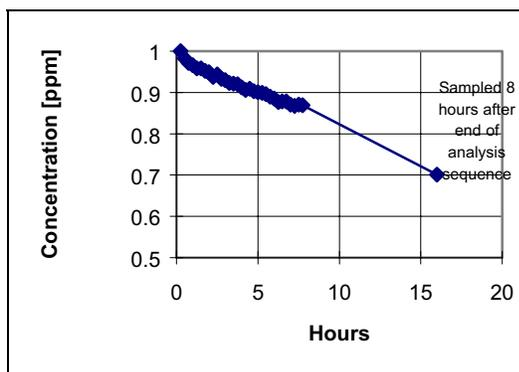
Figure 40 Gas Bag Effect as Measured on a 1 ppm Styrene Sample
