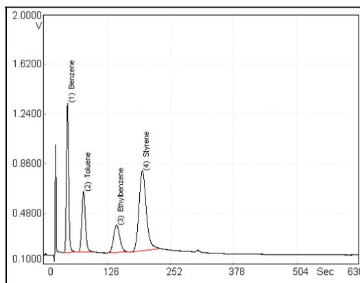
Figure 36 Styrene and Possible Interference Compounds
