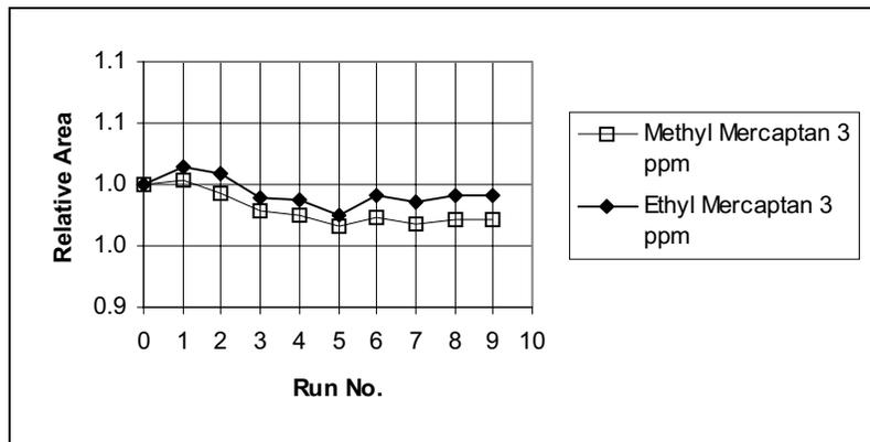
Figure 51 Peak Area Stability for Repetitive Sampling of 3 ppm Methyl Mercaptan and 3 ppm Ethyl Mercaptan
