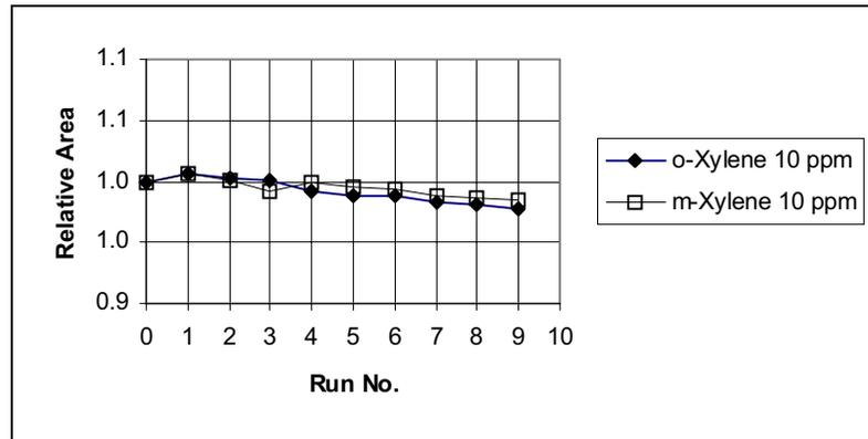
**Figure 33 Peak Area Stability for Repetitive Sampling of 10 ppm m-Xylene and 10 ppm o-Xylene**
