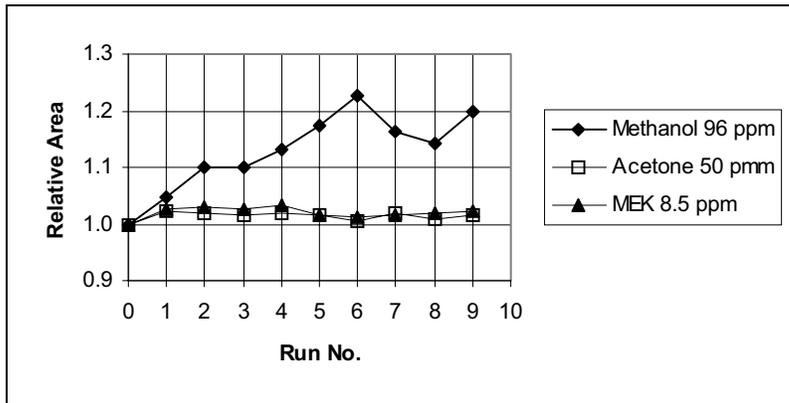
Figure 50 Peak Area Stability for Repetitive Sampling of 96 ppm Methanol, 50 ppm Acetone and 8.5 ppm MEK
