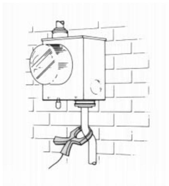
Figure 4-6. Inductive Signal Clamp Hookup
