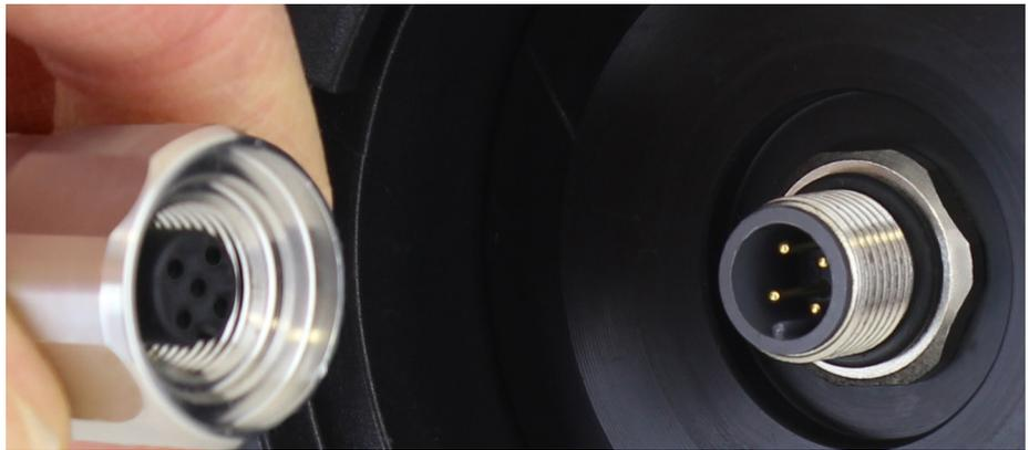
Once properly aligned, carefully push the connectors together, using your thumbs as guides.
