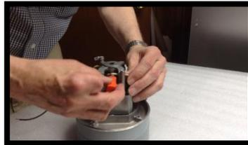
7. Push brush carbon against commutator until plastic brush housing falls into place on commutator end bracket.
