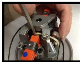
5. With a screwdriver remove brush holder and release **TE-33384** brushes.
