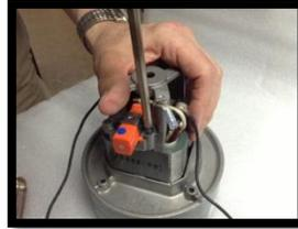
6. With new **TE-33384** brushes, carefully slide quick disconnect tabs firmly into tab slot until seated.
