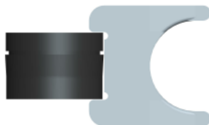
Figure 6-7 Checking Filter Holder to confirm that it is Fully Closed
