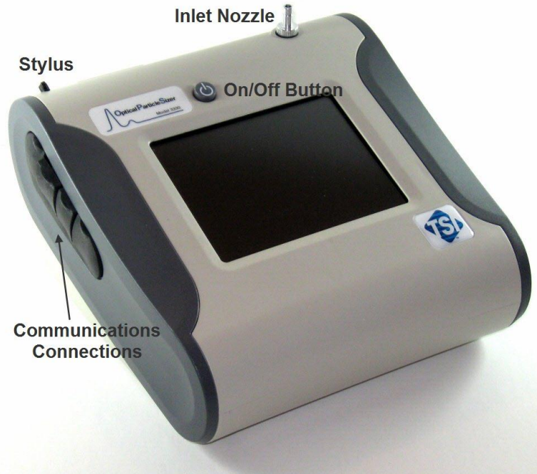
Figure 3-1 Model 3330 OPS Spectrometer Components Showing Inlet Nozzle, On/Off Button, Stylus, and Communications Connections
