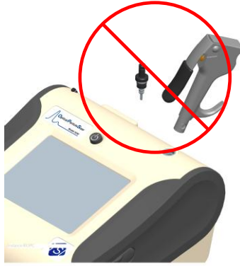
Figure 6-2 Do NOT Blow into the Instrument.
