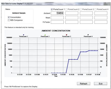
FitPro+ software begins by instructing the PortaCount Pro Respirator Fit Tester to take an ambient concentration reading and store the value. Then the PortaCount Pro Fit Tester begins continuous monitoring of the mask concentration.
