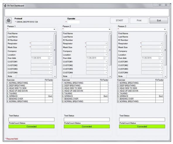
The fields can generally be filled out as normal. However, for those users operating the model 8038, all test subjects must use a respirator of similar efficiency (N95 or N99). A Mixture of N95 and N99 respirators cannot be tested at the same time because the protocol timings vary.
