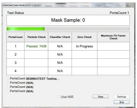
2. If you are using a PortaCount Fit Tester that supports N95 testing and plan to fit test filtering facepiece respirators that are less than 99% efficiency, you must select the "Use N95" box. If you plan to fit test respirators with >99% efficiencies AND <99% efficiencies, you should run two Daily Checks, one with the "Use N95" box checked and the other with the box unchecked.</p>
