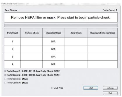
As the test progresses, status messages and additional instructions will be displayed for this unit. When the test completes, the next PortaCount Fit Tester to be checked will be displayed above the instruction field.
