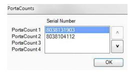
**Note:** If using a PortaCount Fit Tester with version 2.9 firmware or greater, a lock screen should appear on the PortaCount Fit Tester display. Older firmware will not show the lock screen. This lock screen indicates the PortaCount Fit Tester number which makes it easy to coordinate the instruments.
