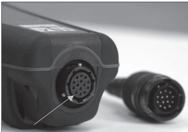
Figure 3, Note the keyed connector.
